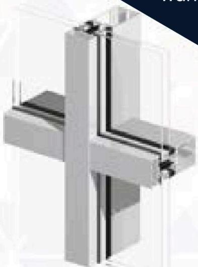
Glazed aluminium curtain wall components are manufactured off-site and delivered for installation. The system, including glass and accessories, is assembled on site using mullion-drained and pressure-equalised principles. Perimeter sealing is achieved using EPDM gaskets and wet-applied silicones, with scaffolding, mast climbers, or scissor lifts required for installation.
